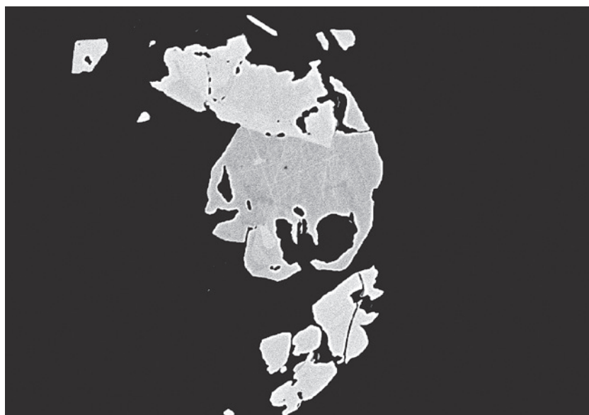
Fig 7 Grains of cassiterite (top and bottom grains light grey, points 159, 160; middle grain darker grey, points 156, 157) in arsenopyrite (black) of sample ST 414 E2. Field of view 300 \mu\text{m} . BSE image of polished section ST 414 E2.
