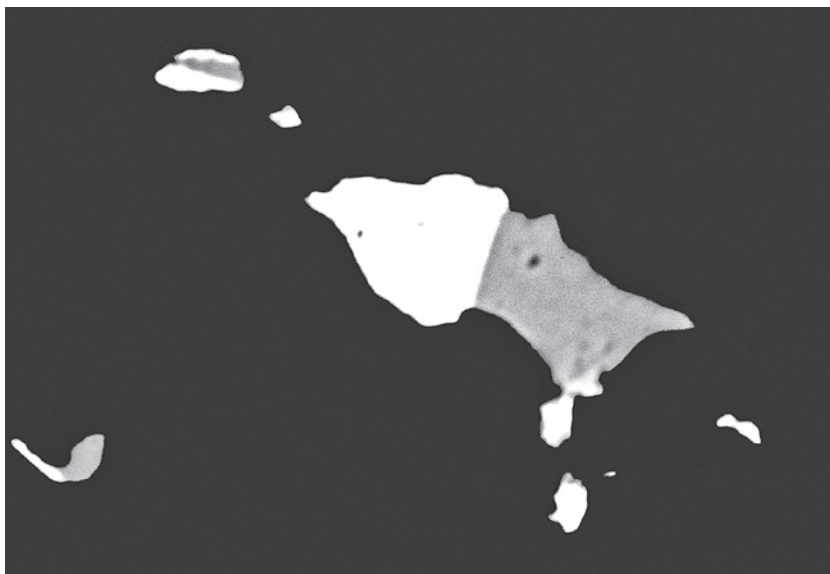
Fig 1 A grain of dantopaite (grey) and native bismuth (white) in arsenopyrite (black). Field of view 75 \mu\text{m} . BSE image of polished section ST 414 E2.
